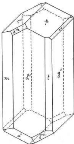
FIG. 7. A typical crystal of sodium molybdo-tellurate showing the ten principal forms, the usual prismatic habit, and a tendency towards pseudo tetragonal symmetry. (Horizontal plan and clinographic projection in the standard position:  $18^{\circ}30'$  rotation and  $9^{\circ}30'$  tilt. Drawn from the stereographic projection VI, Fig. 6.)
