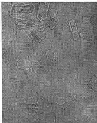
FIG. 1. ( \times ca. 130 diameters). Euhedral crystals of dickite mounted in Canada balsam. The crystals are slightly out of focus so as to bring the Becke line just within the crystal boundary, thus emphasizing the outline.
