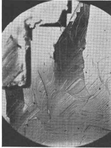
FIG. 5. Photomicrograph of galena cleavage surface, \times 43 . This photograph was taken with normal illumination using a metallographic microscope, with the cleavage surface tipped slightly so as to give a maximum contrast between several lineages. The parent crystal stock is at the bottom of the photograph. Between a quarter and half way up, this splits into four branches, a dark one at the left, another dark one in the center, and alternating light ones. Degree of illumination is a measure of degree of deviation from the parent orientation. This illustration is especially introduced to indicate the derivation of the central dark lineage from the parent stock and its gradual change in orientation. The square motif is the cubic cleavage traces. The fine lines on the surface will be discussed in a later paper.
