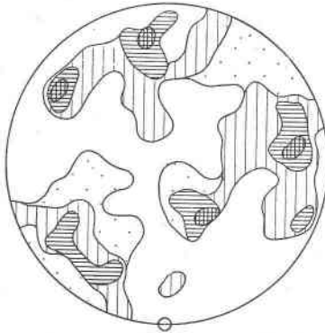
FIG. 8. Orientation diagram for 145 quartz grains in several shadows in the same thin-section. The plane of projection is the plane of rock cleavage. The small circle designates the pole of the Streckung .
