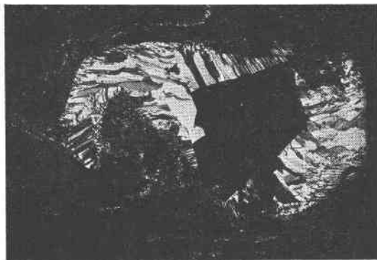
FIG. 2. Distorted "pressure-shadow" with feather quartz in various orientations. Crossed nicols. \times 11 .
