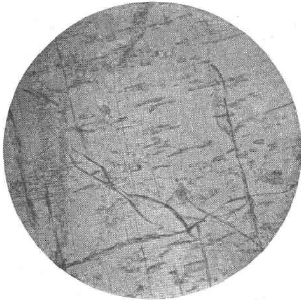
FIG. 5. Rhodonite from Långban (Specimen 2), section about perpendicular to (001) and (110), and showing traces of the cleavage according to the latter face. In the rhodonite a few isolated and irregularly bounded grains of diopside are present. Furthermore numerous smaller, lamellar inclusions of the same mineral are visible arranged parallel to (001). To the left a fissure like line is seen along which the diopside-"perthite"-inclusions are abundant. Magn. 48 \times , crossed nicols.
