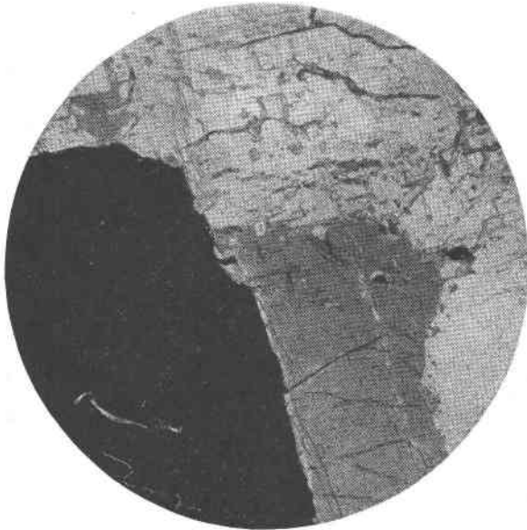
FIG. 3. Rhodonite (white) and bustamite (dark) graphically intergrown with each other. The small inclusions of a lamellar or tabular shape, occurring above the greater part of the bustamite, consist of diopside-perthite. The more irregular, partly ramified inclusions in the rhodonite in the upper part of the figure and to the right of the greater part of bustamite consist of calcite. Magn. 28 \times , crossed nicols.
