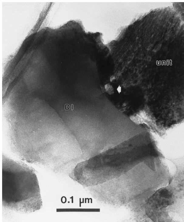
FIGURE 2. TEM micrograph of aggregate IDP L2011K7 showing the interface between a single crystal of diopside (DI) and a ferromagnesian silica matrix unit with a large vesicle at the interface (white arrow). Lineation in the unit probably indicates heating close to its melting point followed by rapid quenching.
