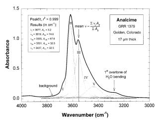
**FIGURE 1.** The infrared absorption spectrum of a 17  $\mu$ m thick analcime slab showing the stretching vibrations of the  $H_2O$  molecules. In addition to the background line and the weighted mean wavenumber, the component bands from peak-fitting are indicated by thin lines.
