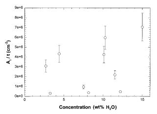
**FIGURE 2.** Integrated intensity  $(A_i)$  of the OH stretching fundamentals (normalized to 1 cm sample thickness) vs. water concentration in weight percent of H<sub>i</sub>O.
