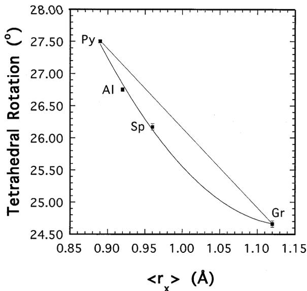
**FIGURE 6.** Plot of the tetrahedral rotation angle,  $\alpha$ , vs. the radius of the X-site cation for synthetic end-member aluminosilicate garnets. The straight line connects pyrope and grossular, and the curved line is a quadratic fit to the data and has no physical significance. The data are from Armbruster et al. (1992) for pyrope, Geiger et al. (1992) for almandine, and Geiger and Armbruster (1997) for spessartine and grossular. The ionic radii are from Shannon (1976).
