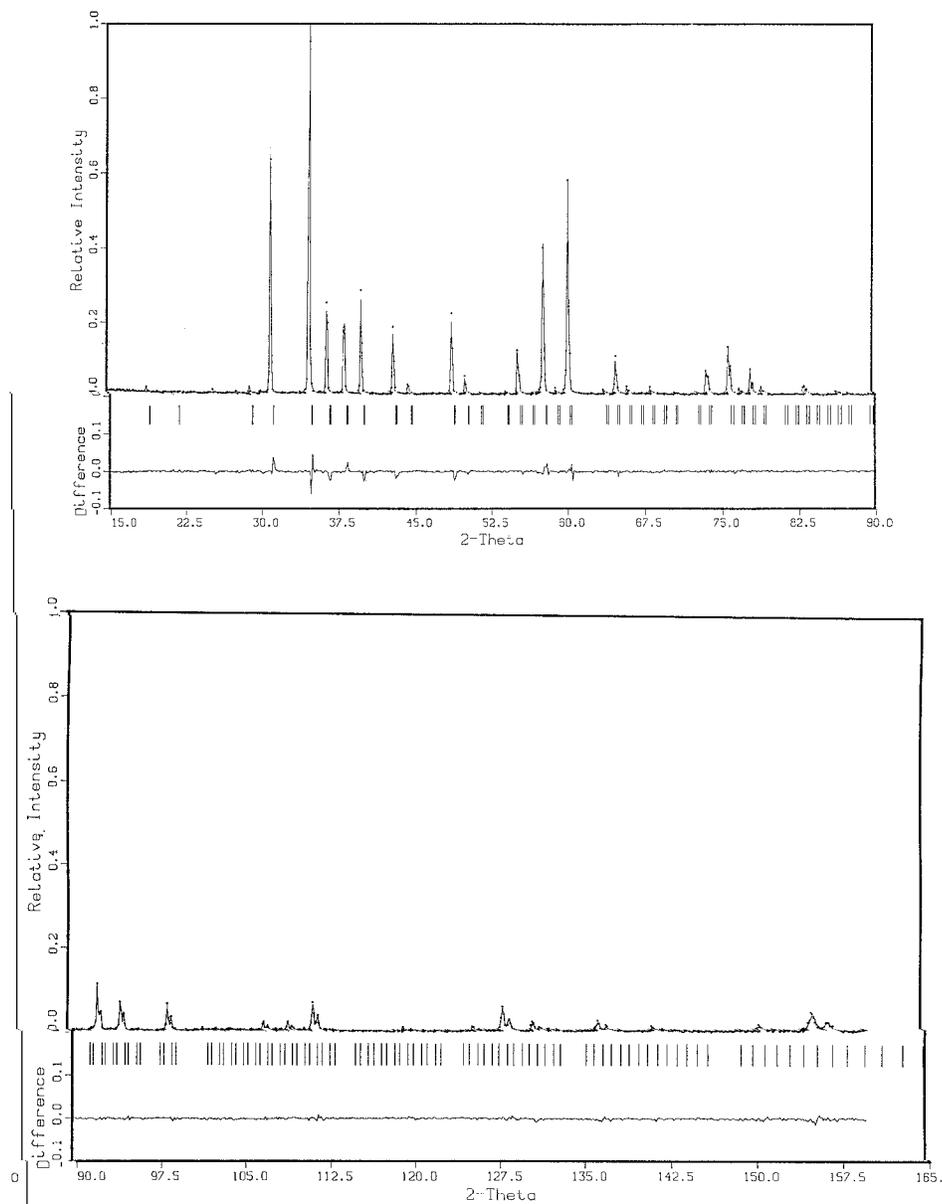
FIGURE 2. Observed (solid points), calculated (best-fit line) and difference plot for garnet of composition  $Py_{75}Al_{25}$ . The positions of all allowed Bragg reflections are indicated as vertical lines directly beneath the profile. The background has been fitted by a fourth-order polynomial.
