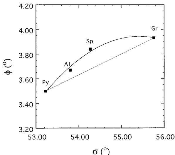
**FIGURE 8.** Plot of dodecahedral distortion ( $\phi$ ) vs. octahedral-tetrahedral distortion ( $\sigma$ ) for the aluminosilicate garnets. The straight line connects pyrope with grossular, and the curved line is a quadratic fit to the data. The sources of the data are the same as those used in Figure 6.
