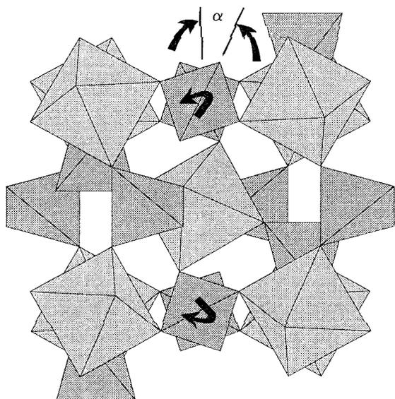
**FIGURE 5.** Polyhedral model of the garnet structure viewed down the  $c$  axis. The corner-linked, rigid tetrahedra and octahedra form a three-dimensional framework. The divalent cations (not shown) occupy the large cavities and are surrounded by eight O atoms in dodecahedral coordination. The arrows in the tetrahedra show rotations to smaller values of  $\alpha$ .
