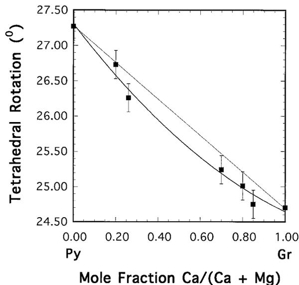
**FIGURE 7.** Plot of the tetrahedral rotation angle,  $\alpha$ , along the join pyrope-grossular. The Rietveld data of Ganguly et al. (1993) were used to calculate  $\alpha$ . The straight line connects pyrope and grossular, and the curved line is a quadratic fit to the data. The error bars give the uncertainties resulting from the errors in the coordinates of the O atom.
