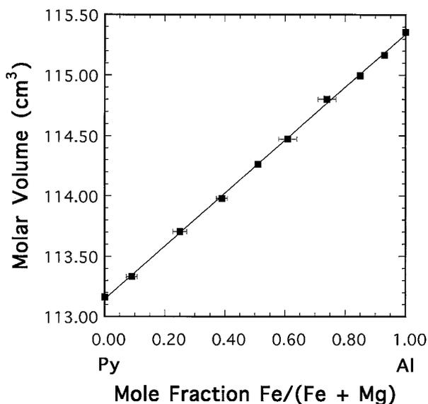
**FIGURE 3.** Molar volumes for the solid solution pyrope-almandine. The solid line is a linear least-squares fit to the data. The error bars represent one standard deviation in the compositions as determined from microprobe analyses. The uncertainties in the molar volumes are smaller than the size of the symbols.
