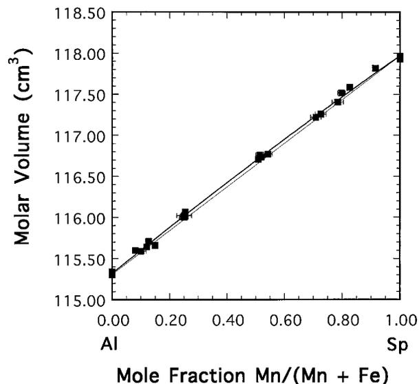
**FIGURE 4.** Molar volumes for the solid solution almandine-spessartine. The upper solid curve gives a least-squares quadratic polynomial fit to the data. The thin line defines ideal mixing between almandine and spessartine. The error bars represent one standard deviation in the compositions as determined from microprobe analyses. The uncertainties in the molar volumes are smaller than the size of the symbols.
