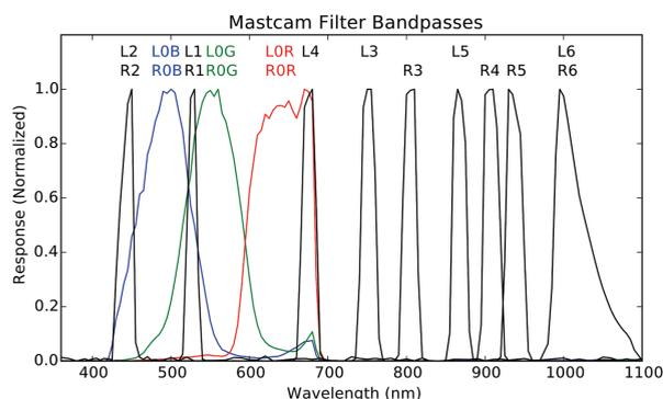
**FIGURE 1.** Mastcam Bayer and narrowband normalized filter profiles for the left and right cameras. The Bayer filter bandpasses (filter 0) are shown in color. For stereo filters, only the left M-34 camera filter profile is plotted, for clarity; the corresponding M-100 profiles are very similar.
