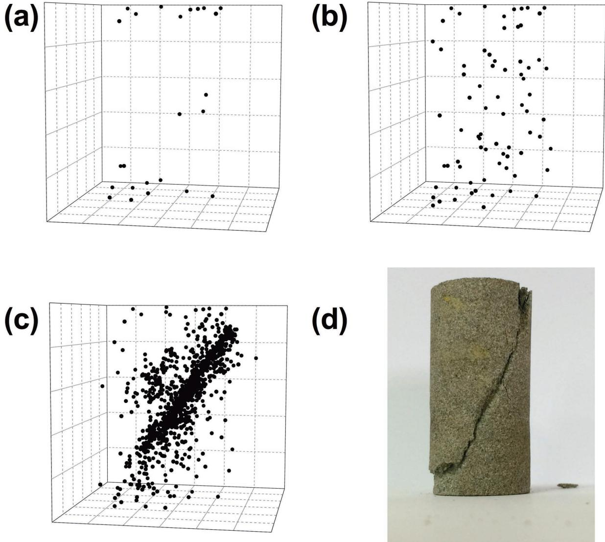
**FIGURE 8.** Evolution of AE centers. (a) A few AE centers appear in the top and bottom areas of sandstone sample from the friction between sample faces and the loading device, (b) some AE centers occur randomly, (c) AE centers form the final crack, and (d) photo of the cracked sample.
