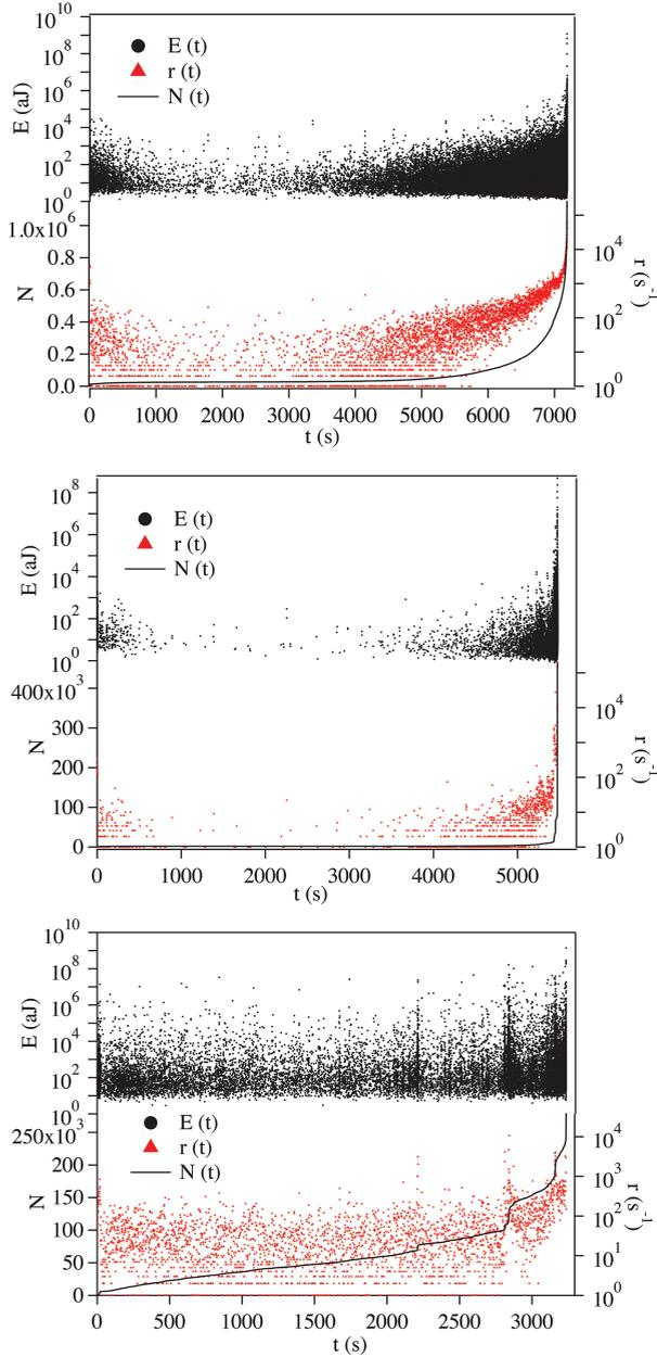
**FIGURE 2.** The energy of the AE signals, the time evolution of the AE activity ( $s^{-1}$ ), and the accumulated number of events for (a) dry sandstone, (b) wet sandstone, and (c) coal samples. In all cases does the activity strongly increase prior to the main failure event. This signal can be used as early warning sign for impending collapse, e.g., in coal mines and buildings.
