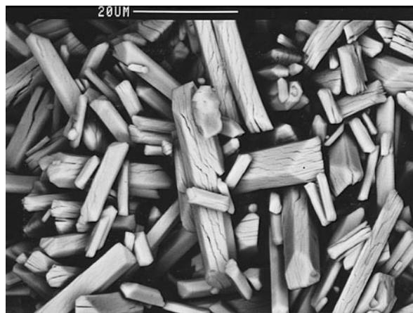
FIGURE 2. SEM photomicrograph of part of a georgeericksenite aggregate: scale bar = 20 \mu\text{m} , note the cracking of the crystals due to \text{H}_2\text{O} loss under the SEM vacuum.
