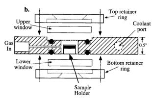
**FIGURE 1.** Schematic diagram of the pressurized optical cell. (a) Top view showing stainless steel body of cell with central, cylindrical sample chamber. (b) Side view showing upper and lower  $SiO_2$  glass windows with o-ring seals and steel retainer rings. The sample holder is a small, cylindrical cup into which water is placed. It is topped by a water-impermeable, gas-permeable layer of hydrocarbon liquid. In both parts bolt holes were left out for clarity.
