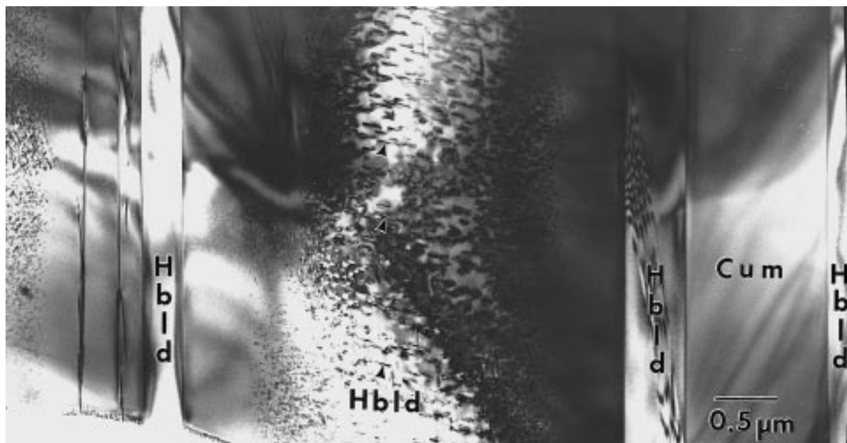
FIGURE 1. A TEM image that shows the cummingtonite (Cum) host and two distinct hornblende (Hbl) lamellar systems. Note that all single-phase regions are well below the spatial resolution of EMA (about 1.5 \mu\text{m} ). Image is taken in non-zone axis orientation.
