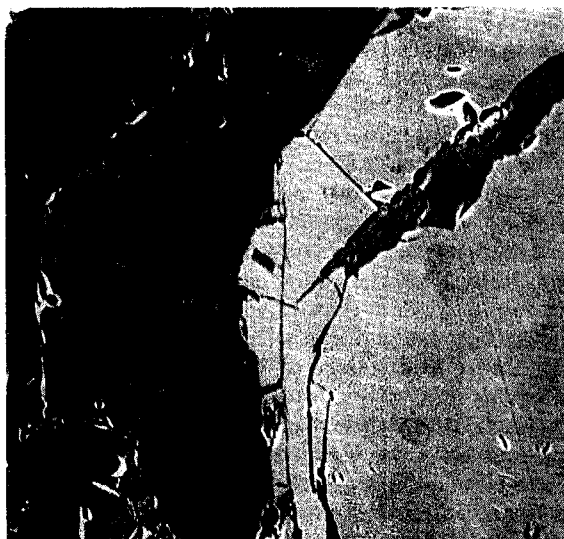
FIGURE 1. Backscattered electron image of the overgrowth of spessartine-grossular garnet on an almandine core. The thickness of the overgrowth is \sim 200 \mu\text{m} .
