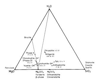
Fig. 1. Selected phases of the system MgO-SiO<sub>2</sub>-H<sub>2</sub>O (MSH) synthesized at pressures below 100 kbar. The molar ratios of MgO:SiO<sub>2</sub>:H<sub>2</sub>O are given in parentheses.
