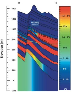
FIGURE 7. Zeolite distribution in an east-west cross section ( $4\times$  vertical exaggeration), approximately defined by drill hole USW H-6 to the west and UE25b no. 1 to the east. Approximate depth and location of the repository host horizon (transparent box) and the SWL (yellow-green line) are indicated for reference. Zeolite scale on the right-hand side of the figure is set so that abundances  $\geq$ 20% are shown as 20% (red).
