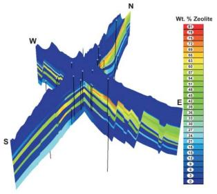
**FIGURE 9.** Three-dimensional cross section of the zeolite distribution at Yucca Mountain, cut off at the base of the Tram Tuff. N-S branch is an expanded version of Figure 6, and the E-W branch is an expanded version of Figure 7. Locations of drill holes within the cross section are indicated by vertical black lines. Note that the zeolite scale ranges from 0 to 80 wt% (red).
