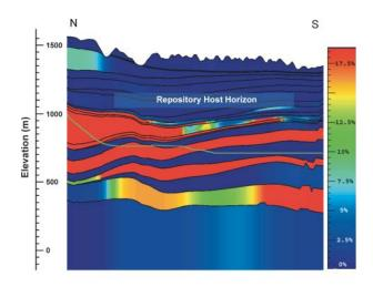
FIGURE 6. Zeolite distribution in a north-south cross section ( $4\times$  vertical exaggeration), approximately defined by drill holes USW G-2 to the north and G-3 to the south. Approximate depth and location of the repository host horizon (light-blue box) and the SWL (yellow-green line) are indicated for reference. Zeolite scale on the right-hand side of the figure is set so that abundances  $\geq 20$  are shown as 20% (red).
