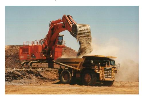
Figure 6; loading ore at Wodgina mine, Australia.
