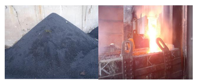
Figure 5: A pile of tantalum rich tin slag, and its treatment. (Pictures courtesy Malaysia Smelting Corporation)
