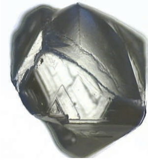
Figure 13. A 2–3 mm partially dissolved (resorbed) pseudo-hemimorphic South African diamond displaying a dodecahedroid top and pristine octahedral lower portion. [Image by Jeff Harris.]
