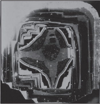
Figure 20. A clear 2.4 mm coated octahedron with an internal growth patterns of what became known as center-cross diamonds, now known as mixed-habit or cubo-octahedral diamonds. [Republished with permission of The Royal Society (U.K.), from Growth history of a natural octahedral diamond. Harrison ER, Tolansky S (1964) Proc R Soc London A 279:490–496; permission conveyed through Copyright Clearance Center, Inc.]
