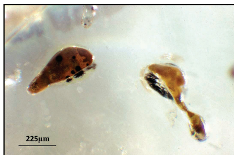
Figure 57. Two inclusions with the typical features of varying shape, as well as graphite on inclusion interfaces and in stress fractures. However, after X-ray analyses, both crystals were identified as powdered goethite, probably pseudomorphs after olivine or enstatite. Inclusions are in a diamond from Ghana. [Image by Jeff Harris.]
