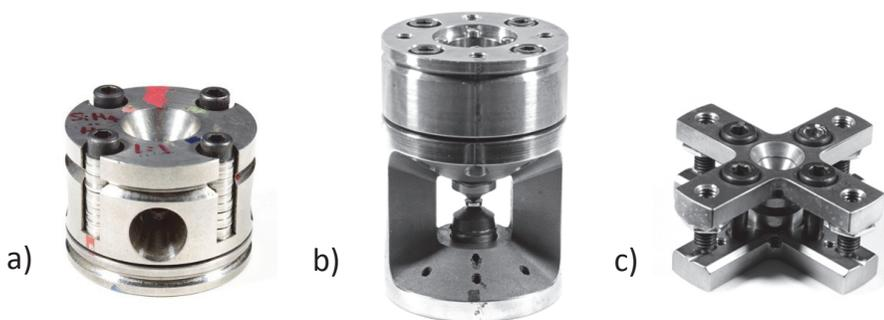
**Figure 2.** (a) Symmetric DAC; (b) Panoramic DAC with radial access; (c) cross DAC with radial access and axial access.
