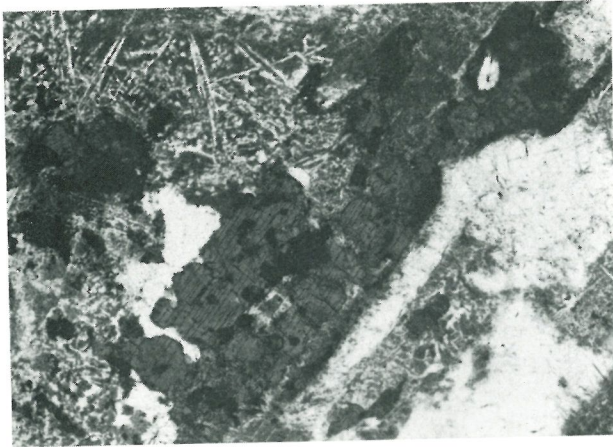
FIG. 4. Photomicrograph of specimen EG 3021, showing acicular crystals of quartz that are believed to have inverted from tridymite. Anhedral quartz crystals, products of direct precipitation from the magma, are also present in his specimen. Reproduced by kind permission of the Clarendon Press, Oxford. \times 20 .
