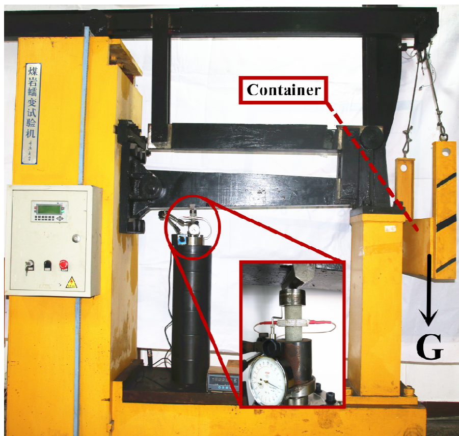
567 FIGURE 1. Photograph representation of the compression arrangement.
