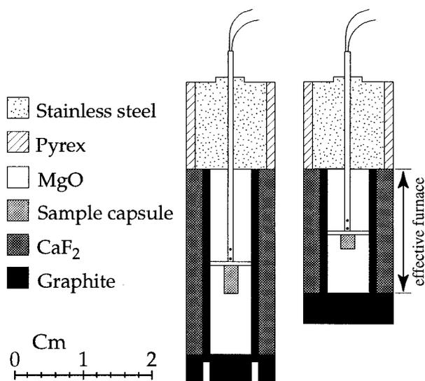
**FIGURE 2.** Cross section of pre- and post-experiment 1.27 cm (1/2 in.) furnace assemblies. Drawn to scale, the illustration at right is typical of the average 30% overall shortening we see in our experiments carried out at 10 kbar. Note the compaction of the lower graphite parts to accommodate furnace extrusion, which is discussed in the text.
