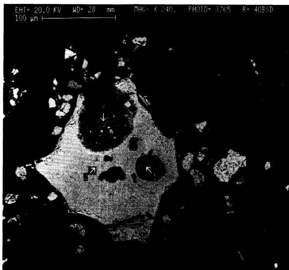
Fig. 2. Scanning electron micrograph showing a grain of Mg-rich maghemite (2) with anatase inclusion (1) and an associated silicate (3).
