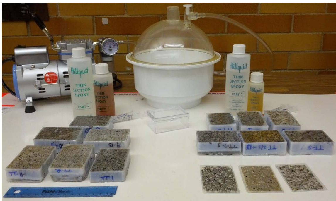
Figure 1. Sample preparation equipment and examples of impregnated lava dome samples and thick sections.
