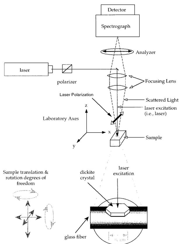
**FIGURE 2.** Schematic diagram of the Raman spectrograph showing the laser, polarizer, optics, sample orientation, analyzer, spectrograph, as well as the laboratory axes. An expanded view of the sample stage shows the dickite crystal attracted to the glass fiber by electrostatic attraction. The sample stage had  $xyz$  translation and rotation about  $x$  and  $z$ .
