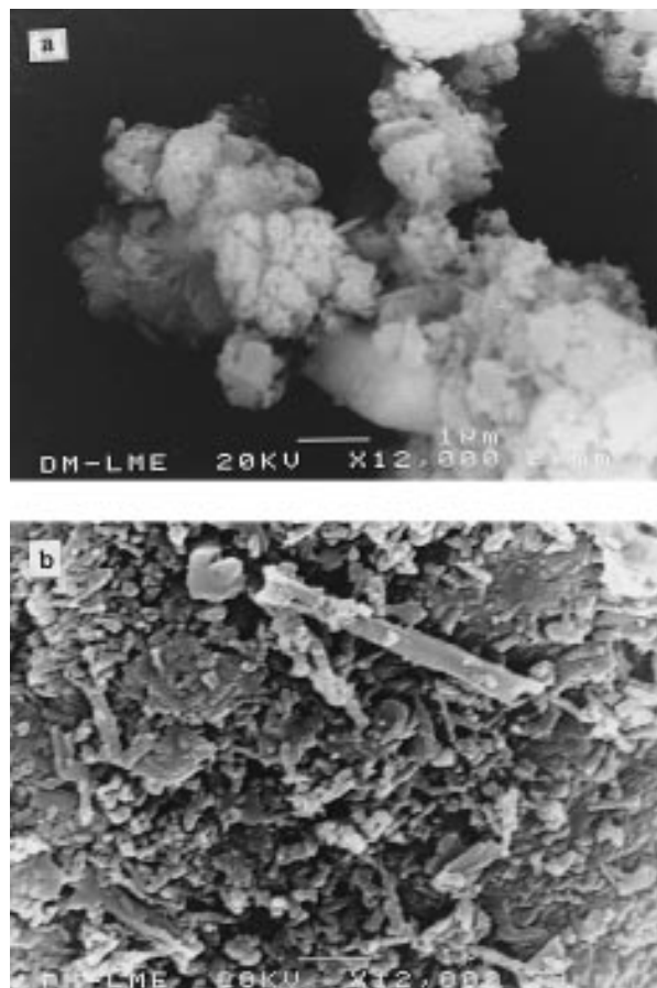
FIGURE 5. (a) Calcium rich dolomite. (b) HCMC fiber-like forms.
