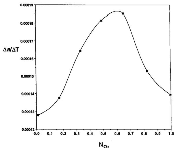
FIGURE 2. Slope of the  $a$  unit-cell dimension with temperature from Figure 1 plotted as a function of mole fraction  $\text{KAlSi}_3\text{O}_8$  ( $N_{\text{Or}}$ ). The curve is interpolated and is not a least-squares fit.
