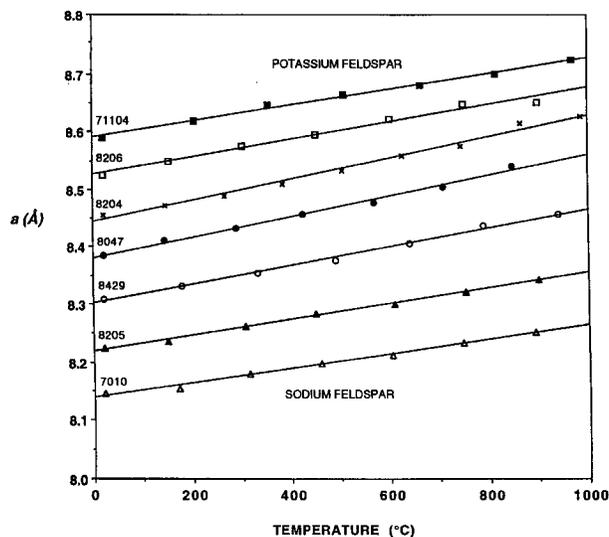
FIGURE 1. Plot of the  $a$  unit-cell dimension vs. temperature for the designated feldspars. Slopes of the lines are shown in Figure 2.
