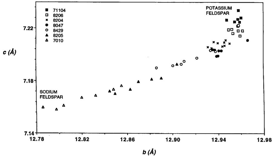
FIGURE 3. Plot of the  $b$  vs.  $c$  unit-cell dimensions of various feldspars. Values increase from lower left to upper right as temperature increases for each feldspar. Note that these parameters expand for sodic feldspars but are essentially constant with temperature for potassic feldspars.
