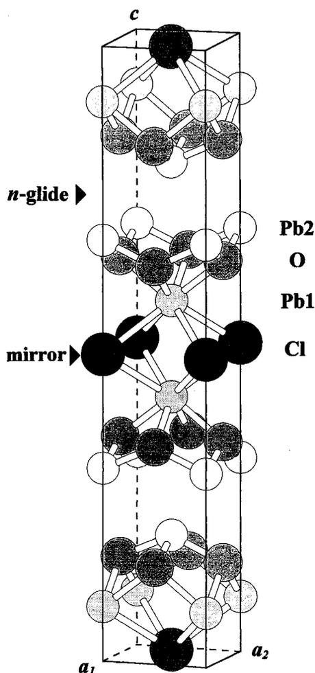
FIGURE 1. The subcell of parkinsonite ( $a = b \approx 4 \text{ \AA}$ ,  $c \approx 22.5 \text{ \AA}$ ). Pb1 sites are light gray, Pb2 sites are white, O sites are medium gray, and Cl sites are dark gray. The stacking module is Pb2-O-Pb1-Cl-Pb1-O-Pb2. The basic building block is the strongly bonded unit between  $n$  glides. The stacking direction is along  $c$  in the tetragonal varieties. The corresponding stacking orientation in monoclinic types is along  $b$ .
