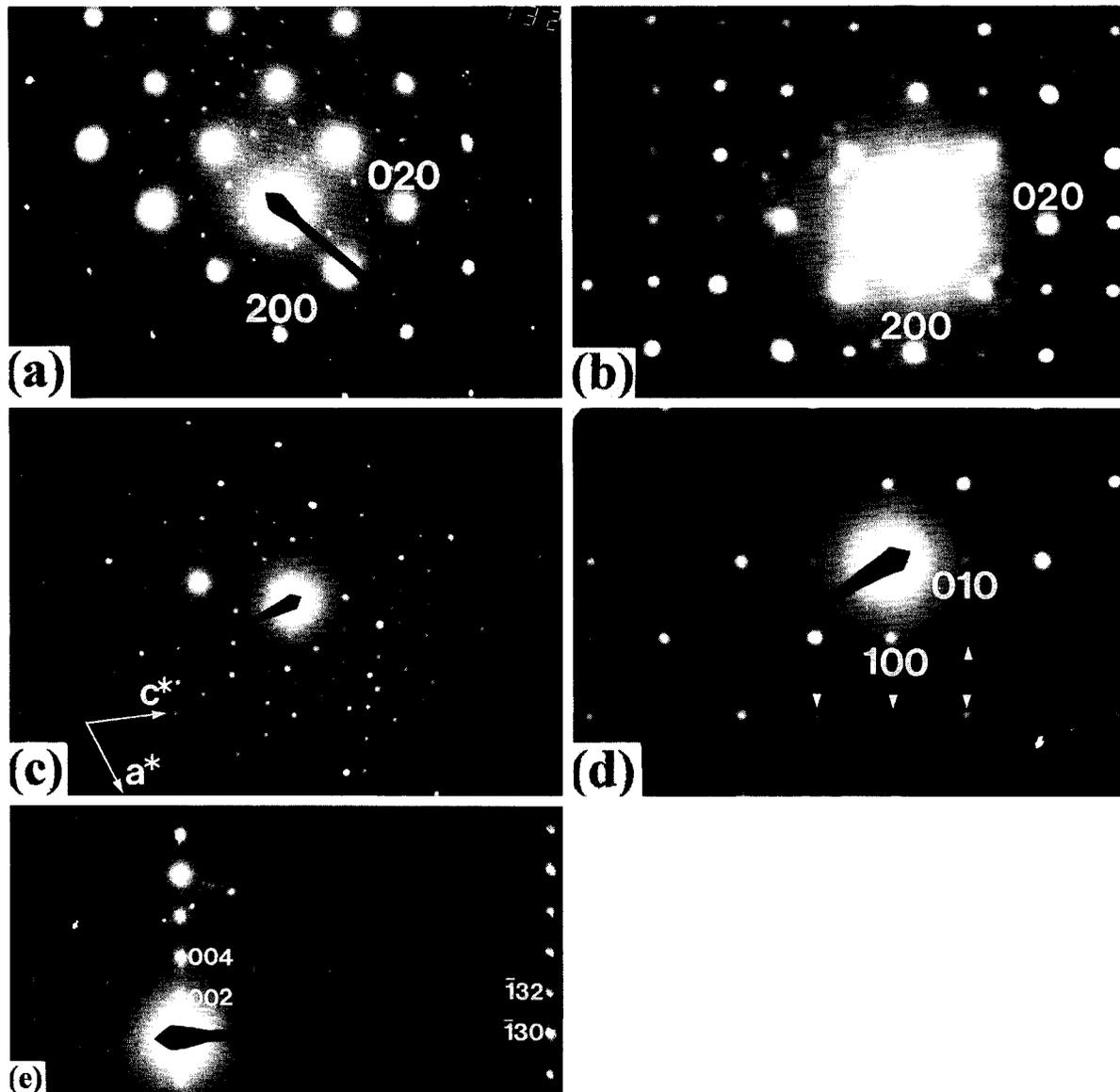
**FIGURE 2.** Parts **a**, **b**, and **d** are the [001] SAEDPs of V-bearing parkinsonite, synthetic parkinsonite ( $\text{Pb}_9\text{MoO}_9\text{Cl}_2$ ), and parkinsonite, respectively. Part **c** is a [010] SAEDP of sahlinitite. All have the electron-beam direction normal to  $\text{PbO}$  sheets in their respective structures. The substructure-superstructure relations are shown in Figure 3. In the SAEDP of parkinsonite (**d**), arrows
