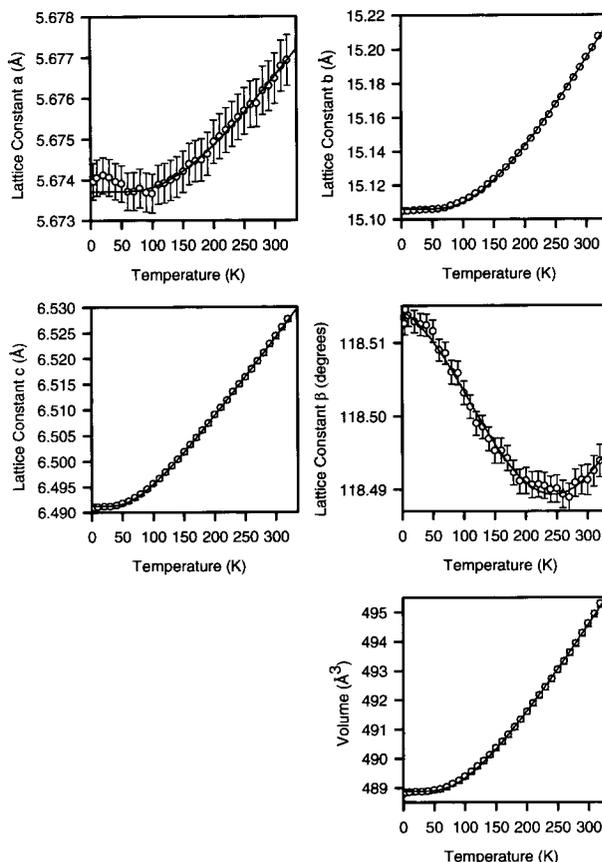
**FIGURE 2.** Variation of the lattice parameters of gypsum within the temperature range 4.2–320 K. The raw data are shown with the calculated fits employing Einstein functions for all parameters except the  $\beta$  angle, which was empirically fitted by a cosine function.
