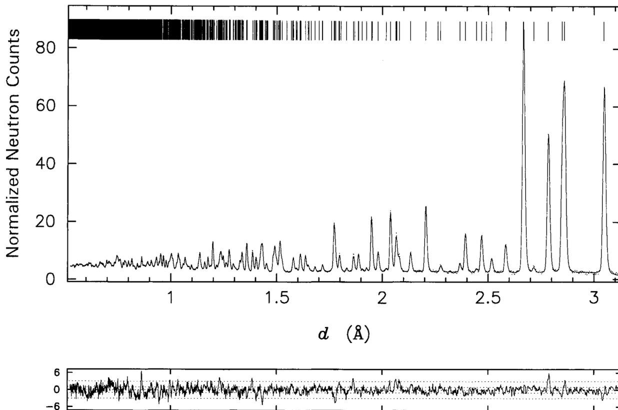
FIGURE 1. Neutron powder diffraction profile of gypsum at 4.2 K. The dots represent the observed data, and the solid line represents the calculated profile. The limits on the residual plot are  $\pm 3\sigma$ .
