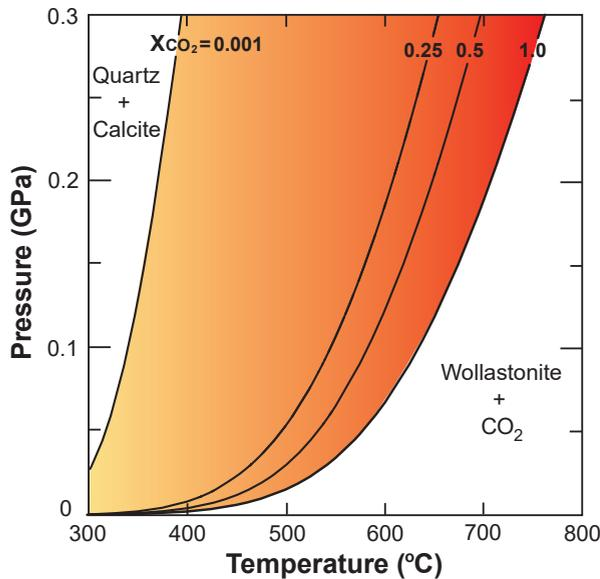
**FIGURE 4.** Pressure-Temperature diagram showing the stability of the assemblage calcite + quartz relative to wollastonite +  $\text{CO}_2$ . Conditions of this reaction are calculated for equilibrium between minerals and fluid of differing  $\text{CO}_2$  content ( $X_{\text{CO}_2}$  is the mole fraction of  $\text{CO}_2$  in fluid). Calculations made using the program Theriak-Domino (de Capitani and Petrakakis 2010) with the Holland and Powell (1998) database.
