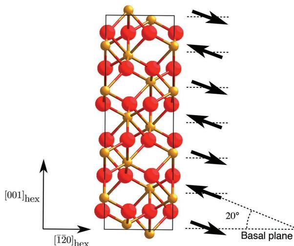
**FIGURE 1.** Crystal and magnetic structure between  $T_M$  and  $T_N$ . The large balls are O atoms and the smaller balls are Fe (or substituted Ti) atoms. The arrows indicate the spin orientation with a  $20^\circ$  tilt away from the basal plane.
