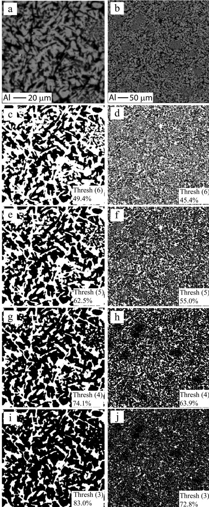
**Supplementary Figure 1.** Threshold testing for two different scales of AlK $\alpha$  X ray maps indicate that the difference small changes in image threshold can have an influence on calculated crystallinities (left column = 100  $\mu\text{m}^2$ ; right column = 500  $\mu\text{m}^2$ ). Threshold value and calculated proportion of crystals (black) are indicated for each image. Original gray scale images are shown in panels a and b.
