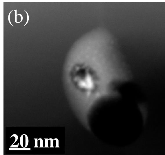
Figure S2. HAADF-STEM images of Pb-rich particle in batch3 (a) and the particle after electron-beam damage (b), revealing that Pb particle is sensitive to the electron beam.
