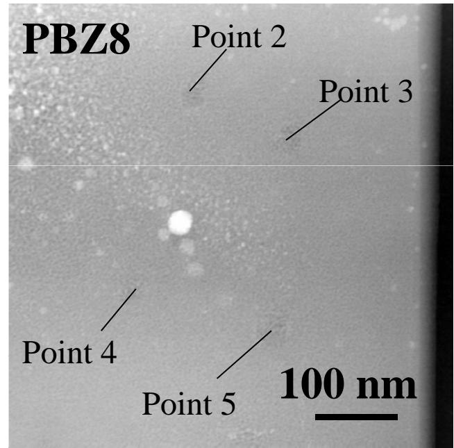
Figure S1. HAADF-STEM images of batch3, PBZ9 and PBZ8 zircon showing the area of the STEM-EDX point analysis for 10 min. of acquisition.
