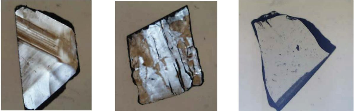
**FIGURE 1.** (Supplementary information) Photos, made under crossed polars, showing the optical properties of the three natural garnets. a.) Gr-44091, b.) Gr-82-112 and c.) Gr-L/K. The platelets range in size from about 2 to 3 mm in cross section.
