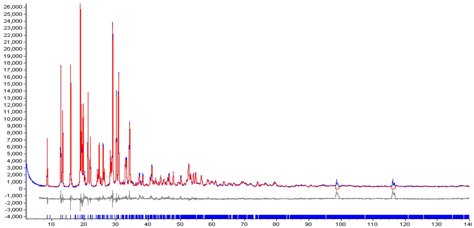
Red, Blue, and gray curves are calculated, measured, and difference curves, respectively. Blue bars are calculated peak positions.
