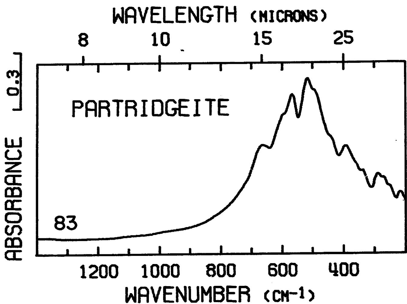
Figure 7A. Infrared spectrum of partridgeite. Presentation intensity: 248%.
