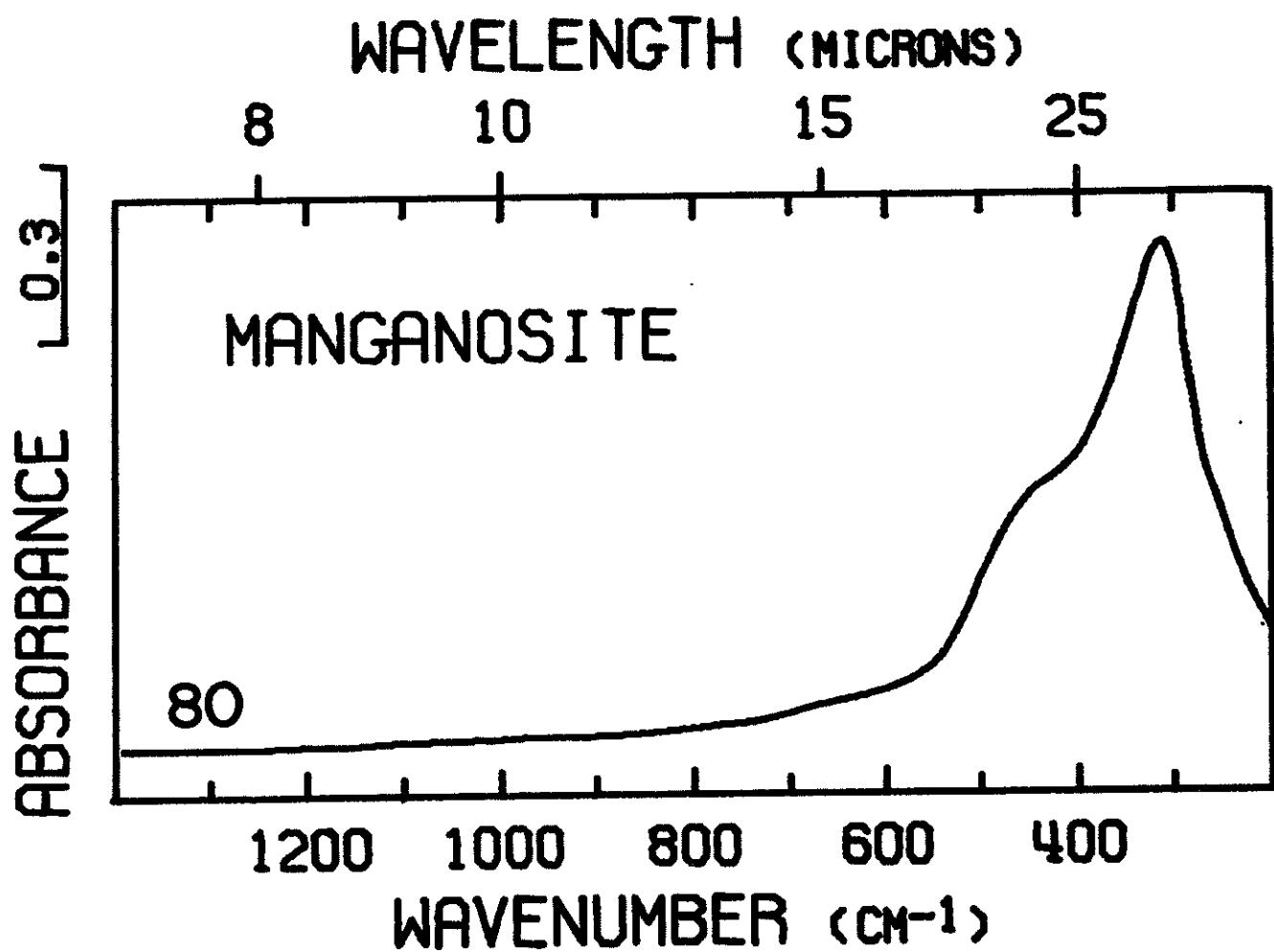
Figure 5A. Infrared spectrum of manganeseite. Presentation intensity: 244%.
