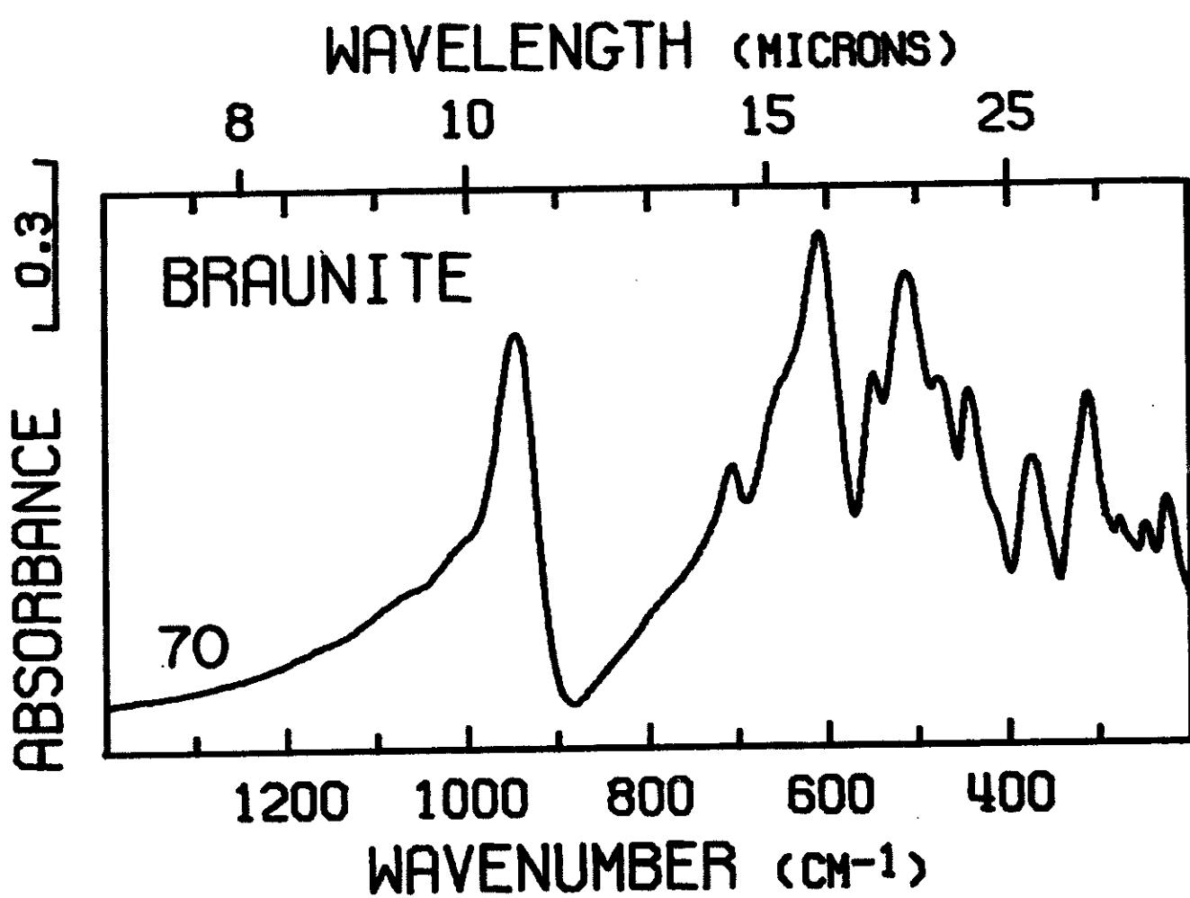
Figure 1A. Infrared spectrum of braunite. Presentation intensity: 344%.
