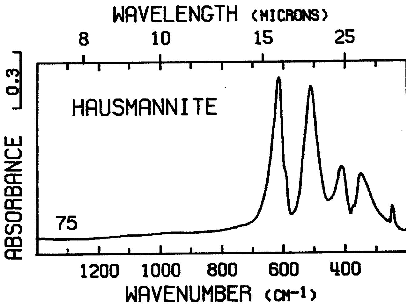
Figure 3A. Infrared spectrum of hausmannite. Presentation intensity: 182%.
