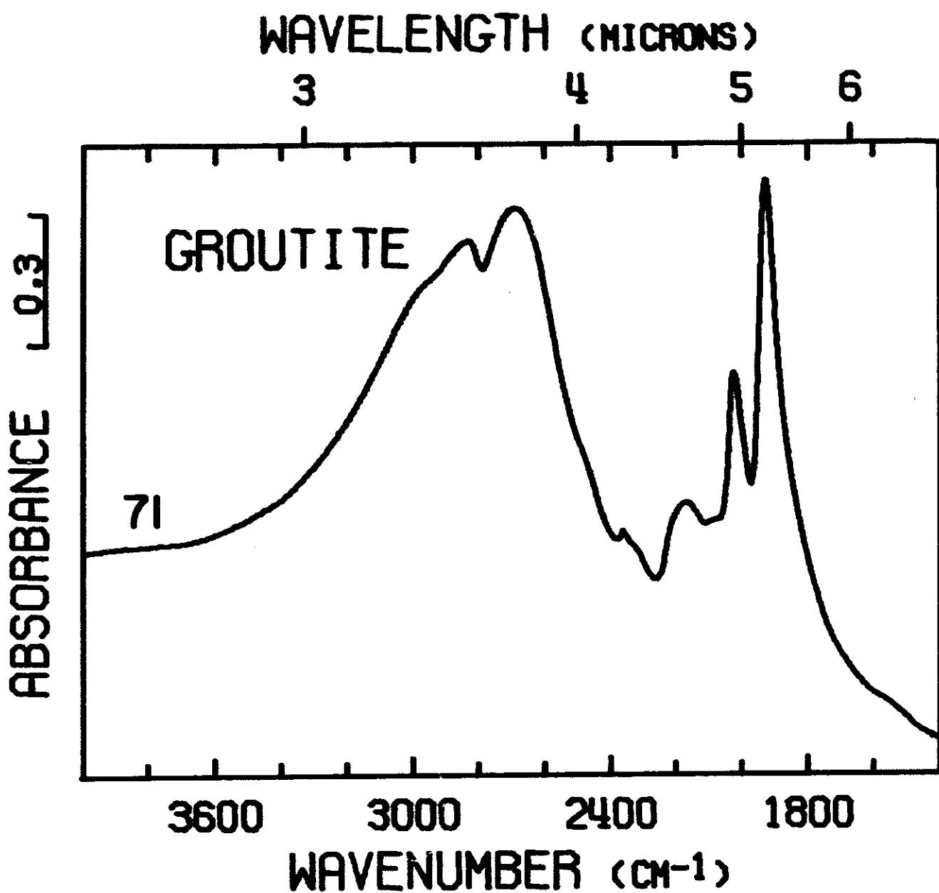
Figure 2A. Infrared spectrum of groutite. Presentation intensity: 268%. Figure continued on following page.
